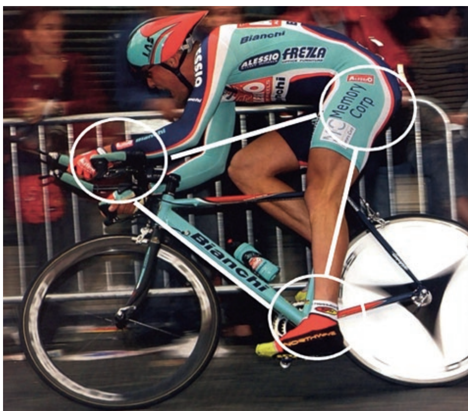
FIGURE 1: The white rings illustrate the three areas of body bike contact, these include the pelvis and buttocks
